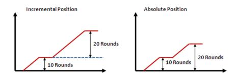
14. Set P2P position command from 04-15 to 04-44. Actually, we have 15 groups P2P position commands and every group has two parameters which are rounds and pulses. MIs status can determine which position group you can use. Please refer to as follows:
