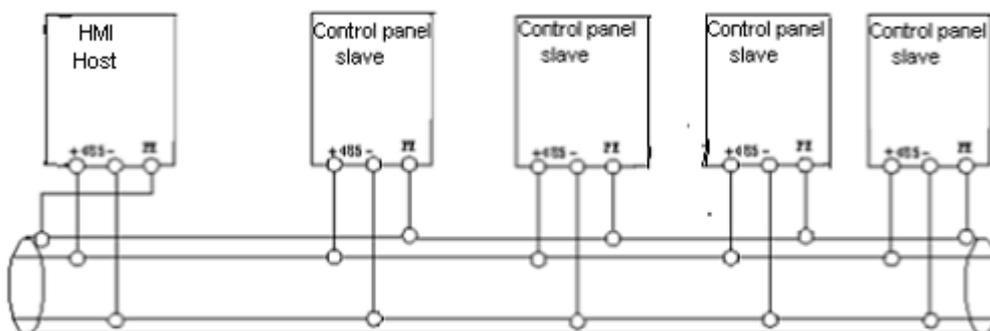
Fourth, the HMI, PLC and inverter communication control, this is suitable for ED3100, ED3200, ED3500, ED3800 series products. But ED3100 will not read (because in the case of reading, there is only one word volume for the data, symbols and unit volume in the ED3100's response frame, please refer to the specific communication protocol of the ED3100 monitoring example), as shown below:
