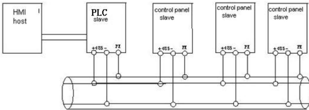
Fifth, PC, IPC and inverter communication control, this applies to ED3100, ED3500, ED3800 series products; This need to install the company developed communication control software interface in the PC or IPC. This communications interface can monitor the inverter operating frequency, output voltage, motor speed, busbar voltage, etc. When using the communication interface, it require to install the VB6.0 or above version to open. As shown below:
