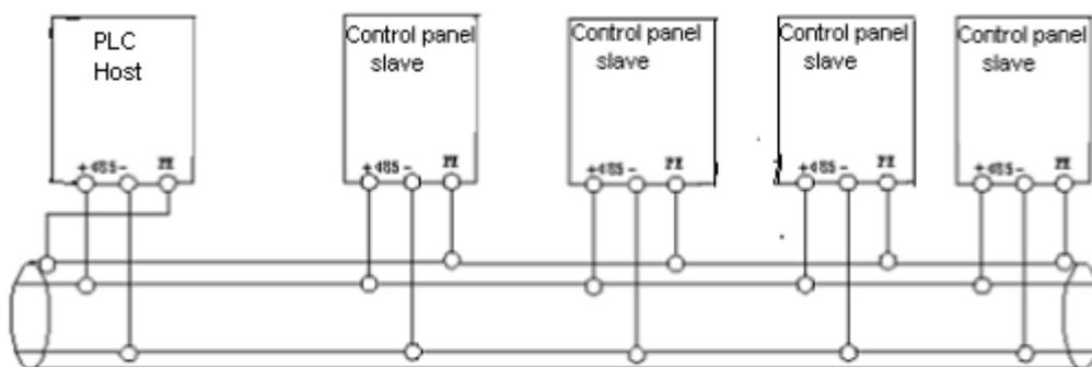
Third, the communication control between HMI and inverter, with this form, the standard MODBUS485 RTU coding mode only suitable for the slave machines of ED3200, ED3500, ED3800 series. As shown below:
