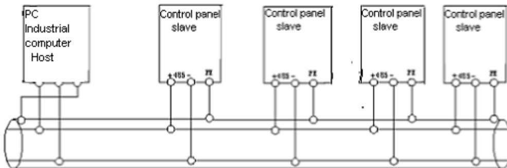
Note: No matter what kind of communication used in the process, can only be between the same series of products to communicate with. Because inverters of different series bear different communication protocols and communication addresses.
